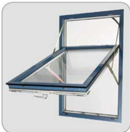
To TURN the window from the TILT position, close the window and turn the handle 90° to the vertically upward position and pull the window inwards. The side remains hinged to the frame whilst the window can be opened inwards to any required position.
